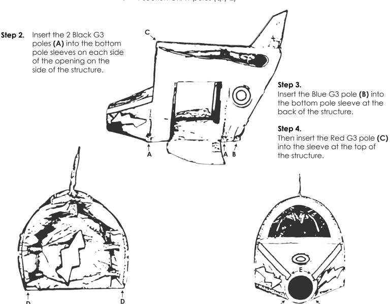
Step 5. Insert the 2 Yellow G3 poles (D) into the bottom pole sleeves on each side of the back of the structure on the bottom.
